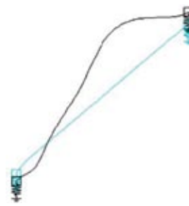
FIGURE 6: First bending mode shape of Keronite/Mg/Keronite cone at f_1 = 15.8\text{kHz} .
