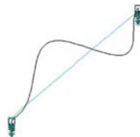
FIGURE 7: Second bending mode shape of Keronite/Mg/Keronite cone at f_2 = 21.9\text{kHz} .
