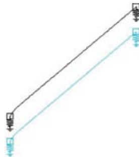
FIGURE 5: Piston mode shape of Keronite/Mg/Keronite moving as-sembly at f_0 = 147\text{Hz} .
