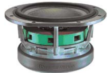
PHOTO 1: B&W 250mm woofer with TEPEX sandwich type Carbon Fiber-TPU/8mm Rohacell 31LS/Carbon Fiber-TPU composite cone.
