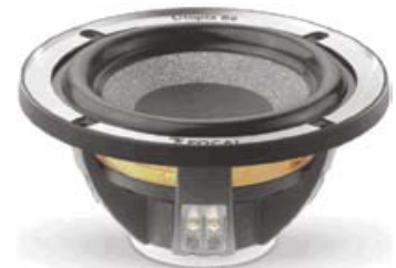
PHOTO 2: Focal 325mm woofer with sandwich type glass fiber-polymer resin/Rohacell/glass fiber-polymer resin composite "W" cone.
