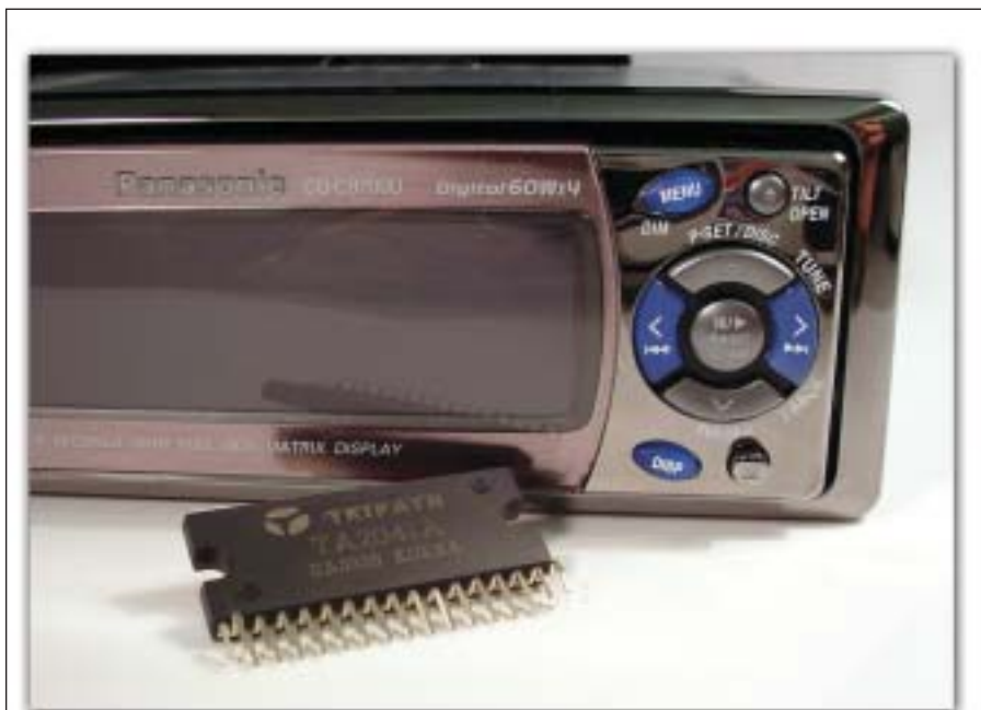
PHOTO 4: Panasonic's car audio head unit with the TA2041 Class T audio amplifier.
